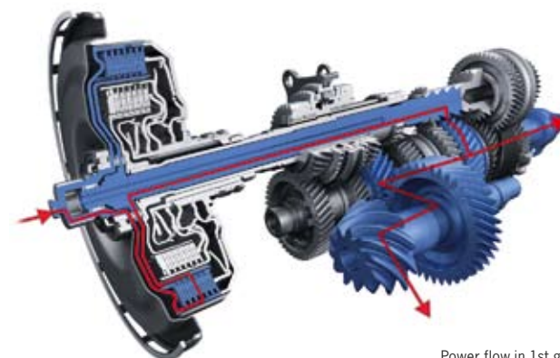
Power flow in 1st gear
